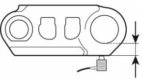
3. To ensure correct measurement is taken, always measure on the inside of the link joins.
