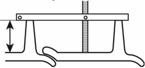
2. Make sure the Depth Gauge is flat against the grouser bar to obtain an accurate reading.
