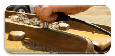
3. If the shoe has been re-barred/re-groused, the Ultrasonic Tool is no longer effective. This is because the signal is interrupted at the point at which the bar has been welded.
