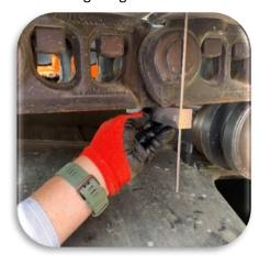
4. Then measure the Pin length exposed using a ruler as demonstrated below.
