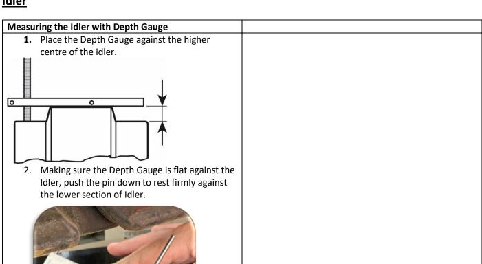
3. Measure the pin length with a ruler or tape measure.
