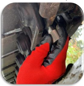
4. If the UT is not returning a reading, gently rotate the probe from left to right until reading is found.
