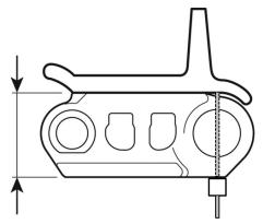
3. Place the depth gauge on the bottom of the rail with pin passing directly through the centre of the bush and touching the under surface of the shoe. This is demonstrated in the following image.
