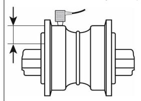
**3.** Place the probe in the centre of the left or right, ensuring probe is making as much even contact with the surface as possible.
