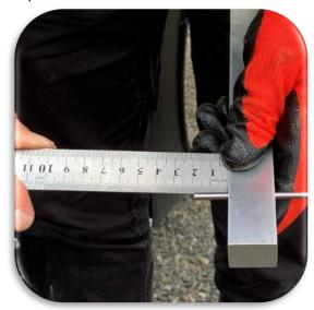
4. Use a ruler or tape measure to measure the pin length.
