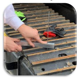
Once the Depth Gauge is flat against the grouser bar, use your free hand to push the pin down to firmly rest against the plate.
